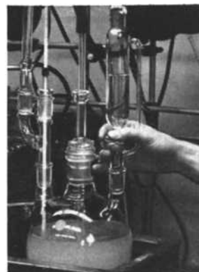
Adding reagents in an epoxidation reaction with hydrogen peroxide.
